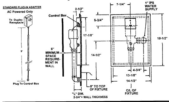
This smooth and quiet concealed flush valve for closet is equipped with adjustable sensor with electronic override button, rough brass finish, solenoid operator, adjustable tailpiece, vacuum breaker, 1" IPS Angle Stop, elbow flush connections, spud connection for 1-1/2" Back Spud. Exposed flush valve parts are chrome plated. Includes Stainless Steel Wall Box and Cover Plate with manual over-ride button.
