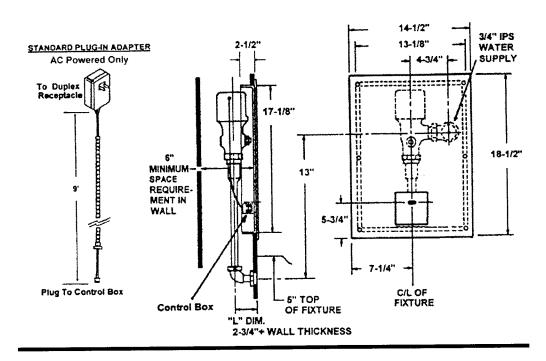
This smooth and quiet concealed flush valve for urinal is equipped with adjustable sensor, rough brass finish, solenoid operator, adjustable tailpiece, vacuum breaker, 3/4" IPS Angle Stop, elbow flush connection, spud connection for 3/4" Back Spud. Exposed flush valve parts are chrome plated. Includes Stainless Steel Wall Box and Cover Plate.
